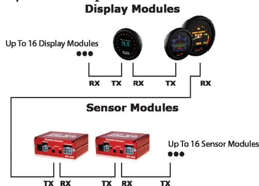
Remove termination jumpers from all sensor modules excluding sensor module furthest from display modules.
